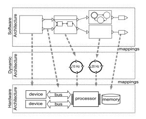
Figure 2. Global view : layers and architecture mappings
